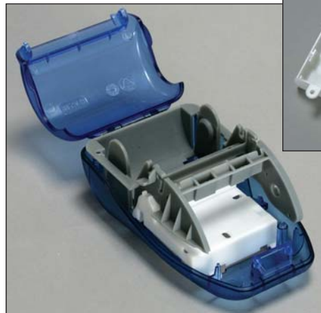
At left: Printer assembly of production (blue) parts and prototypes produced with si 50 grey and natural material
